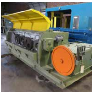
Syncro FX-13 Rod w/Niehoff Annealer, 630 mm Spooler
