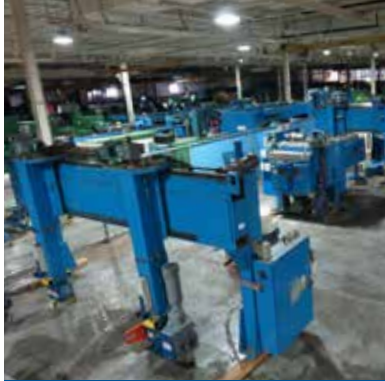
Calmec 2" Interlock Armoring Line
