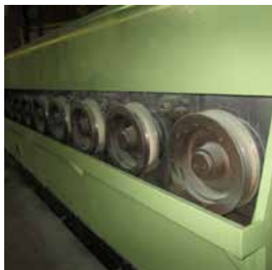
Syncro 18T 10-Die Tandem Rod Line w/ Dual 30" Spooler
