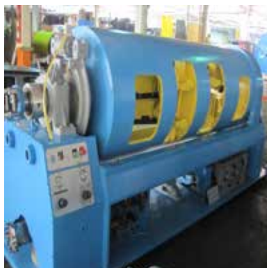
Poutier 72" (1.8m) Rotating Belt Caterpuller
