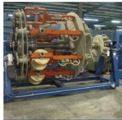
Nokia-Maillefer Fiber Planetary Cabler (15") CBR1001
