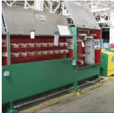
Samp MLS/5,T.14 14-Wire Drawing Machine
