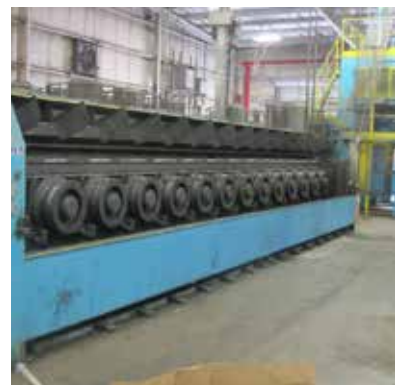
Eurodraw SA450.14.2 14-Die, 2-Wire Rod Breakdown Machine
