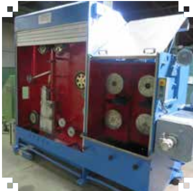
Samp TR/2-TP Wire Drawing Machine
