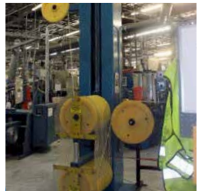
TEC 300' Vertical Accumulator
