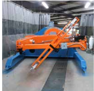
Ceeco Fork Style Drum Twist Line (72")
