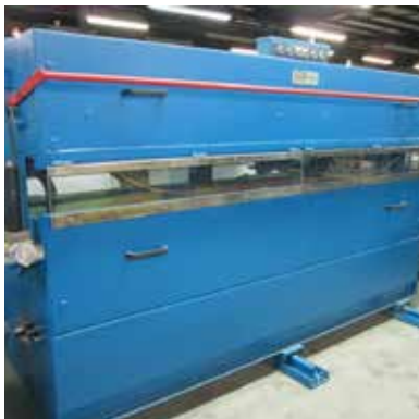
MGS 72" Belt Caterpuller
