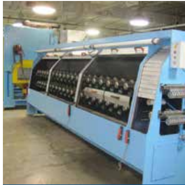
(8) Eurodraw 16-Wire MMS 100.16 SW 800, Drawing Lines
