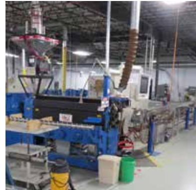
Vitek 3 1/2" Fiber Jacketing Line EXPL416
